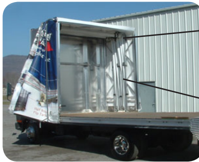
Retracted system showing rolled up rear door and the 100% height clearance that it provides.
