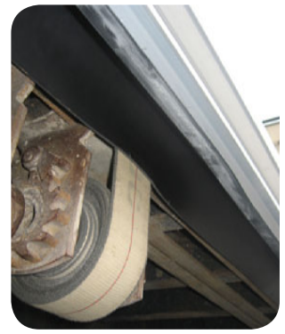
Mudguard bends around straps to keep water and snow out.
