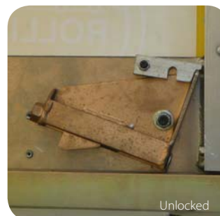
The adjustable rear lock gives you the ability to fine tune your tarp tension.
