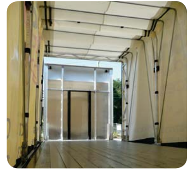
Inside view showing optional double lift bows and standard translucent roof
